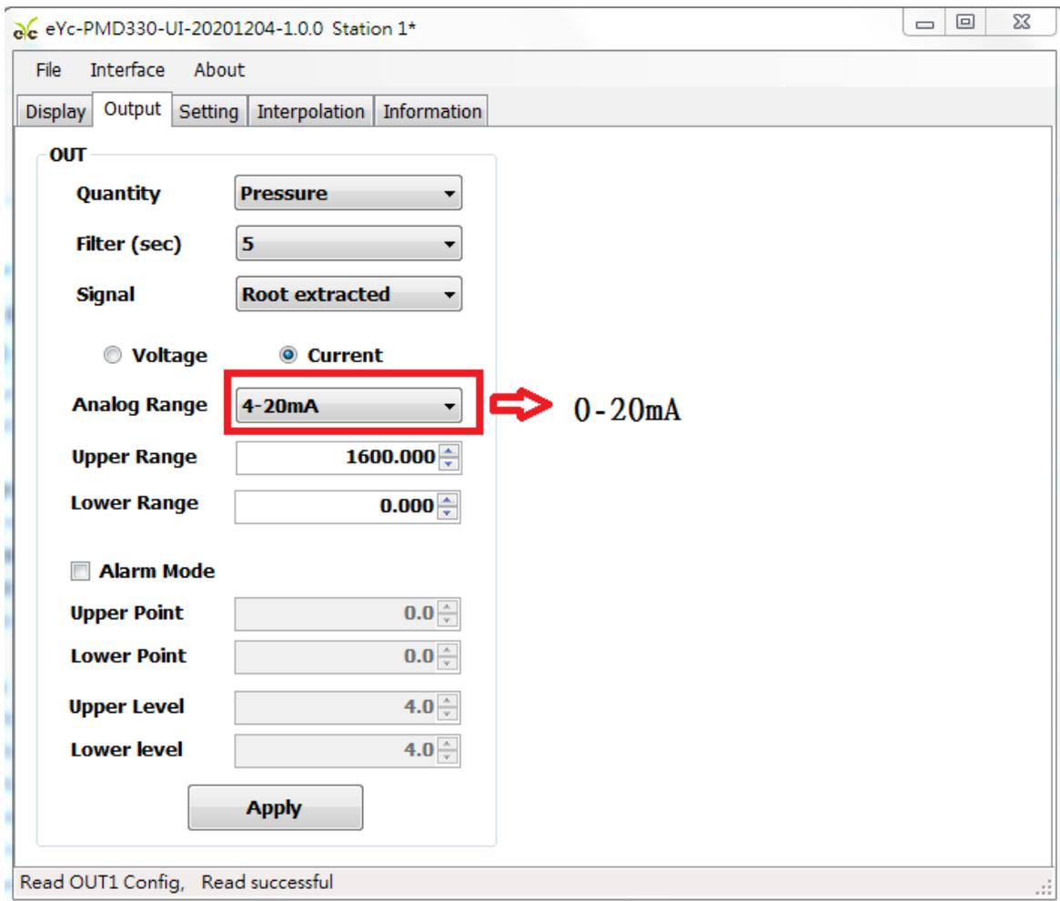
\* If you change the output to 0 ... 10 V, the range setting of UI should also be changed to 0 ... 20 mA.
