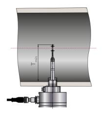
T<sub>min</sub>: Minimum inmersion depth > 58 mm (smaller depth of immersion on inquiry)
